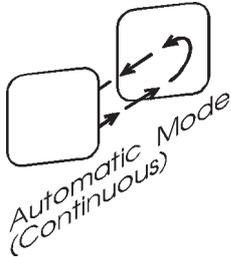
In situations such as exhibitions, a continuously changing colour may be required. This has normally needed a control console to give constantly variable control input to the colour changer. This is a costly solution and also limits the resolution of the fade to the 8-bits of DMX. Mode 8 in the Pluscard allows the user to set up a smooth fade across the complete length of the Gel String, whilst the Rainbow is only supplied with 24 volt DC power.
