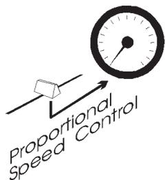
The ability to control the maximum gel speed is important for smooth scrolling between colours and consistently quiet colour changes irrespective of the limits of the incoming DMX control signal. Where required, the processor calculates fades using 12 bit levels which avoids the 'stepping' associated with 8-bit DMX signals. This is especially critical for slow fades on long gel strings and larger colour changers (15", 22", 26" etc)
